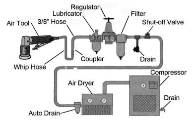
A typical air line layout is shown above. If an automatic in-line filter/regulator is used, it will keep air tools in good condition.
